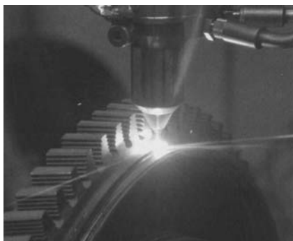
Titanium alloy metal powder guided coaxially to the beam and blown onto the focal point in laser beam buildup welding
