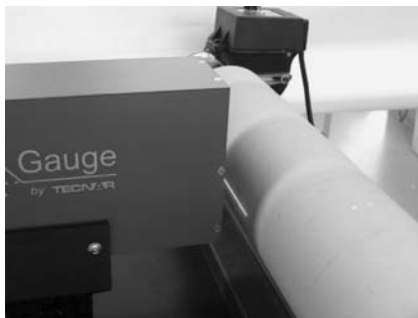
Fig. 2 An optical triangulation-based prototype sensor, LayerGauge, is used for on-line monitoring of the coating thickness deposited per pass. The system resolution is better than 5 \mu\text{m} .
