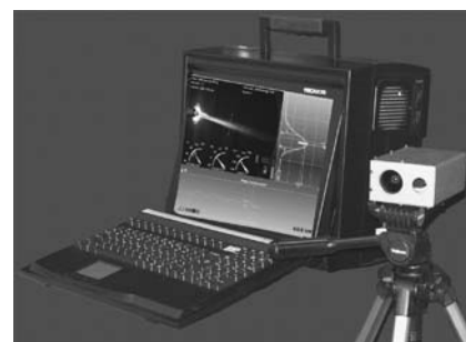
Fig. 1 The AccuraSpray system measures ensemble particle jet parameters (jet orientation, width, and intensity, mean particle temperature and velocity) for monitoring thermal spray processes on the production floor.
